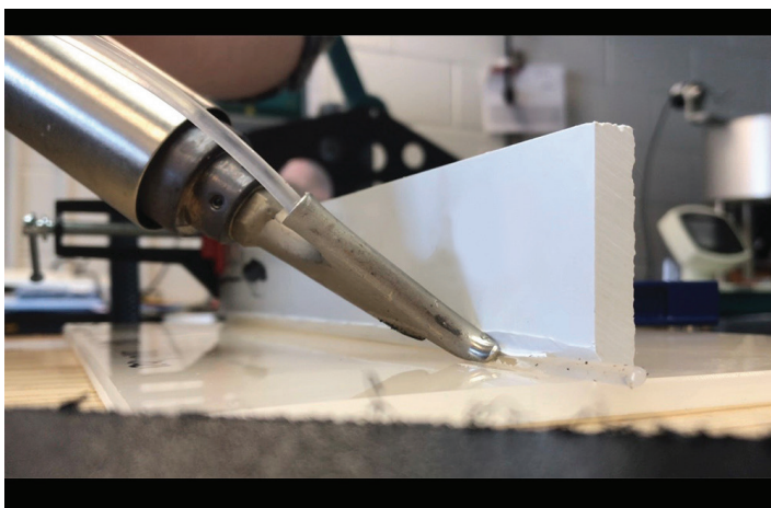
A Wegener hot gas welding gun is used to weld CRP-1.
